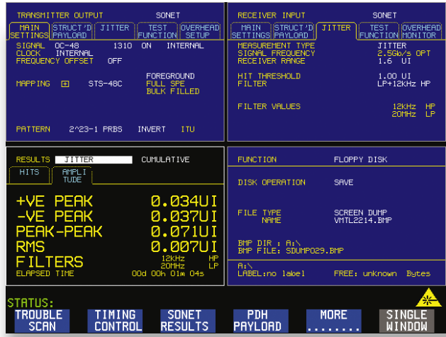
Figure 14. Jitter generation configuration and result (OmniBER 718 screen shot)
