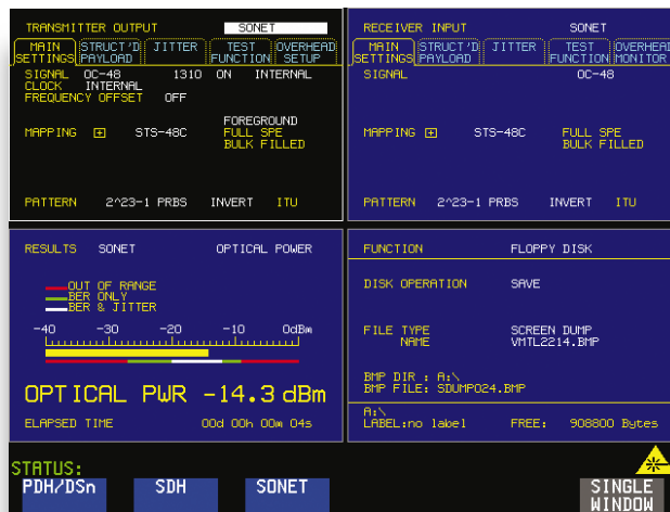
Figure 12. OmniBER 718 screen shot and Rx and TX configuration
